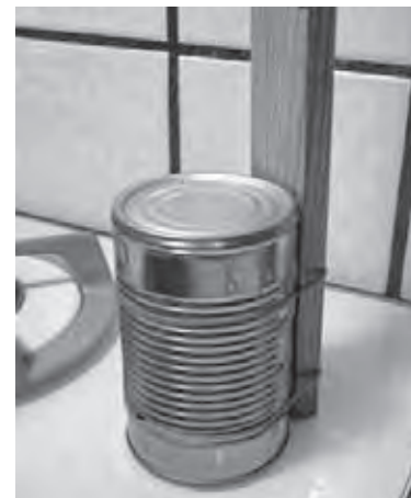
Figure 3. The can and ruler assembly is a model of a geothermal power plant.
